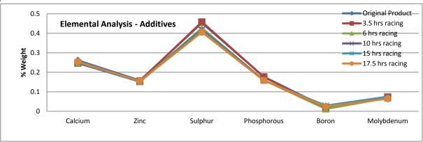
The following graph confirms that the low friction properties of the oil remain the same even after 5 race events.
