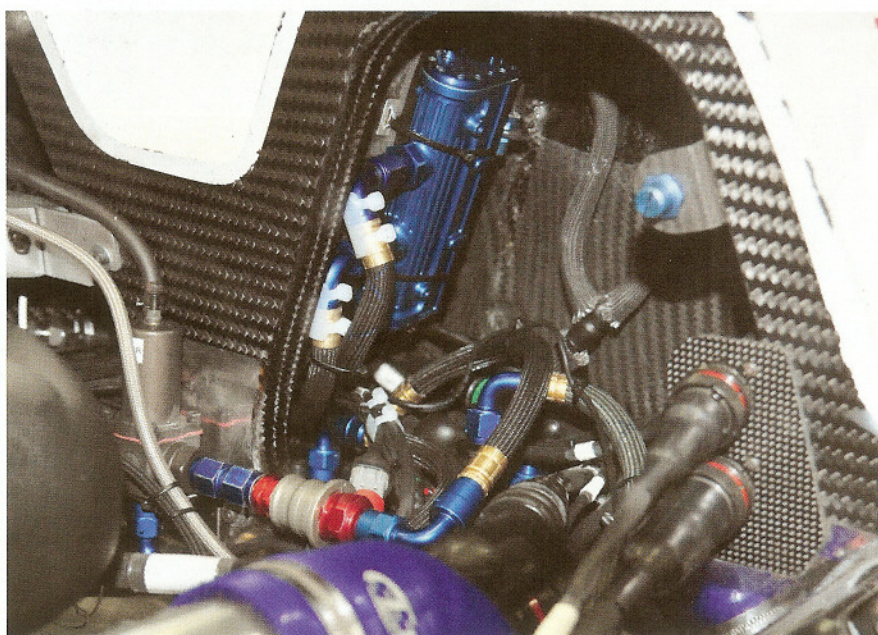
ABOVE & BELOW The Gill Ultrasonic Fuel Flow Sensor (installed in a car, below) offers a glimpse of the future
